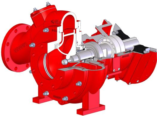
The versatility of portable, automatic priming trash pumps makes them ideally suited for many municipal and industrial sewage and wastewater applications. Selecting a pump with the optimal impeller type - enclosed or open - helps determine the overall field performance and operational cost of the pump.
