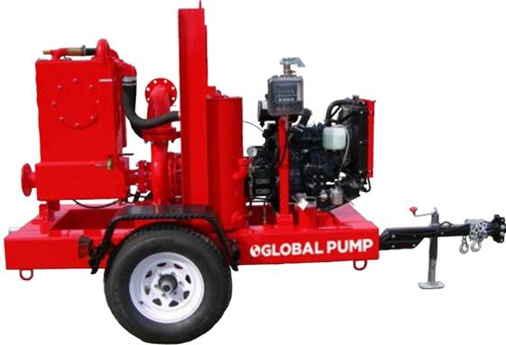
Global Pump® Standard Centrifugal Wellpoint pumps are specifically designed to effectively handle the arduous requirements of wellpoint and underdrain dewatering systems where intermittent water flow and large amounts of air are encountered. The dual diaphragm priming system generates up to 100CFM without the need for an oil-cooled vacuum pump.
